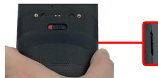
3. Align the battery with the battery compartment, then push forward until you hear a click sound.
