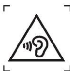
Figure 1 – Warning label (IEC 60417-6044)
